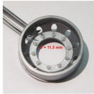
The <u>outer planetary hubs</u> have to be removed completely and the rim's whole has to be drilled up to <u>11,5 mm</u>. It's not required, to change or remove the nuts & bolts from the kit. However, you may exchange them by more detailed ones; in this case consider the wrench size of 22 mm which results into ca. 1 mm in 1/24.
