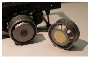
Now both rims should be glued centrically (left picture below). The hub comes either next or omit it for the moment, if rims and hub should get different colours.
