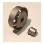
At the <u>inner rim</u> remove the cylinder completely and flatten the surface. For that reason the axle parts have to be cut also, but later on. Consider, that due to this modification the axle does not provide movable wheels any more.
